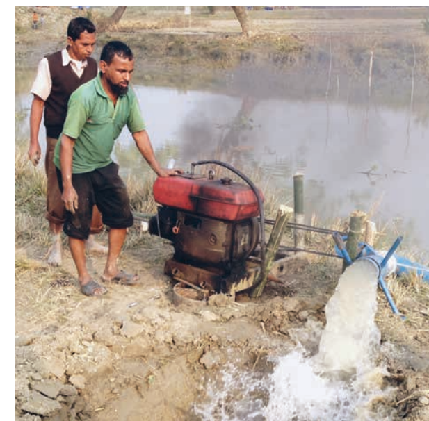
A diesel-powered axial flow pump transfers water from a retention pond in Bangladesh.
