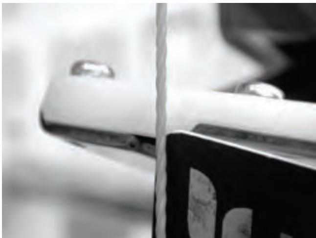
A credit card or drivers license should be able to slide in between the string and the white protective cover (strike plate) without touching the string
