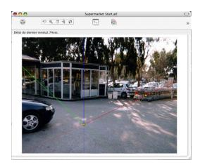
Place the origin of the axis marker on the photo, then pivot the red, green and blue axes one by one.
